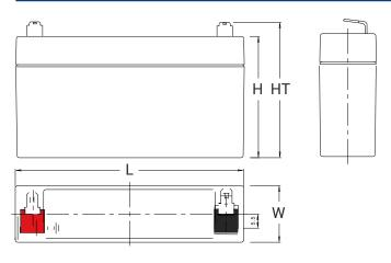
**W:** 0.94 (24) L: 3.81 (97) H: 2.02 (51.5) HT: 2.26 (57.5) Tolerances are +/- 0.04 in. (+/- 1mm) and +/- 0.08 in. (+/- 2mm) for height dimensions. All data subject to change without notice.
